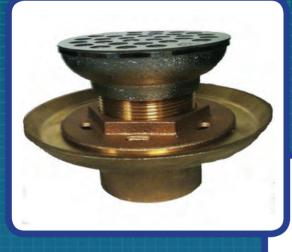
Extra heavy brass body and clamping ring with large surface area to receive pan material. Adjustable chrome-plated cast brass barrel with stainless steel strainer - 3-3/8" center distance on barrel accepts AB&A cast brass round and square strainers. 2" FIP Drain Connection.
