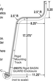
Note to specifier: The BASIN GUARD must be specified in combination with ADA-conforming sinks (example, Elkay GECR or LRAD Line, or Just Manufacturing ADA Line with rear drain) with a maximum 6" deep bowl and rear waste outlet.
