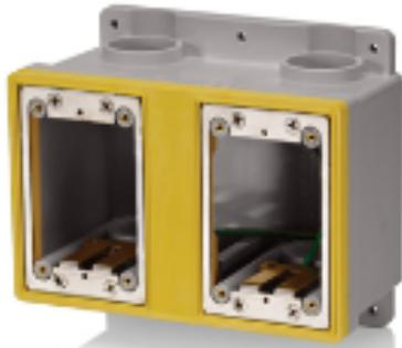
FD Box, Two-Gang, 67.3 Cubic Inch Capacity, 1" unthreaded conduit openings with reducers for 3/4" and 1/2" conduit , includes plugs for unused openings and stainless steel device mounting plates with ground wire, industrial grade - GRAY
