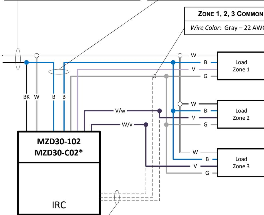
Alternate 0-10Vdc Control Loop Route
