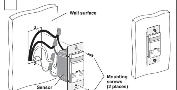
**NOTE:** Dress wires with a bend as shown in diagram to relieve stress when mounting device.
