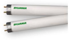
General28W, 48IN MOL, T8 OCTRON Extended Value SUPERSAVER® fluorescentDescription:lamp, 5000K color temperature, rare earth phosphor, 81 CRI, suitable for RS or<br/>IS operation, ECOLOGIC®.
