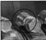
**Mechanical Interlocking Clamp Design:** IDEAL clamps feature a one-piece screw housing that mechanically interlocks the housing to the band. This one-piece housing design eliminates leak paths that can occur in staked or welded clamps.
