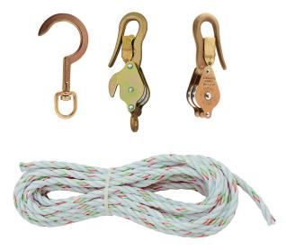
All Klein block and tackle use high-quality, 3/8-Inch (10 mm) diameter rope. Light, galvanized-steel shell blocks are fitted with snubbing hooks to hold the load. This package features two blocks with a swival Klein hook Cat. No. 259 with a maximum safe load of 750-Pound (340 kg).
