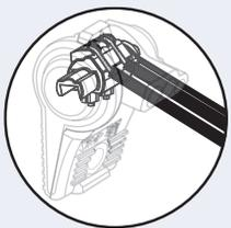
3. Hold wires in place while squeezing handles together until the latch snaps shut.
