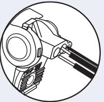
2. Rotate handles fully apart beyond 90 degrees. Insert stripped wires into connector; #12-#14 in the large holes and #16-#20 in the small hole. Exposed ends of wires should be visible through the clear housing on the back.
