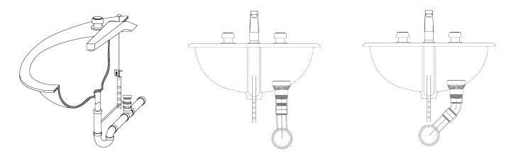
Offset drain waste to avoid conflict between Studor AAV and pop-up drainage linkage
