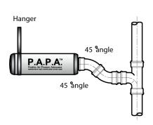
When mounting horizontally (it is advisable to maintain a minimum of a few degrees of slope so as to induce self draining), or at any angle up to 90 degrees, the P.A.P.A. device should be supported or anchored as shown in the left diagram. The portion of the support or anchor in contact with the device housing should allow for expansion and contraction and be rubber lined to prevent damage.
