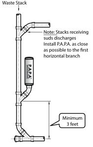
Stack extending more than 5 floors above the base of the stack or offset should be a minimum of 3 feet
