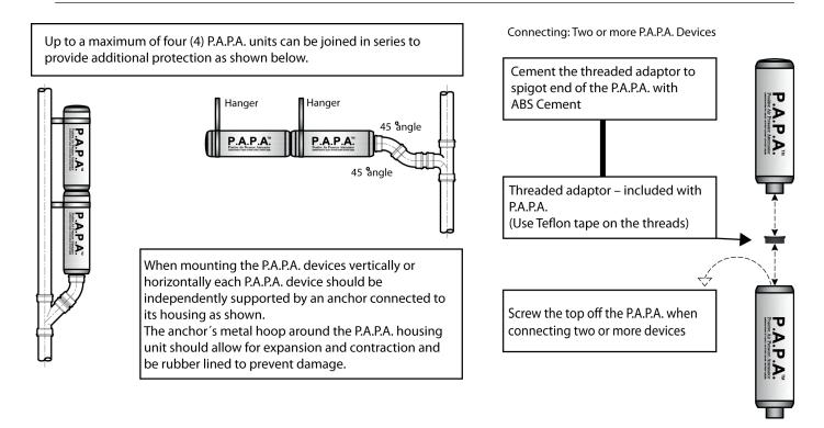
Note: The P.A.P.A. must be installed after the System's pressure test, in an accessible location.
