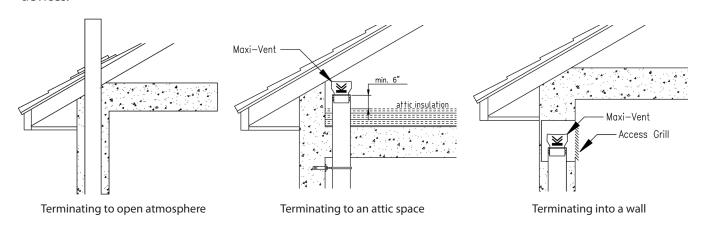
A minimum of one vent pipe shall extended to the open atmosphere for each building drainage system.
