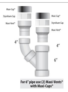
Note: For pipes larger than 6" notify Studor, Inc. Note: Ensure that one open vent is maintained
