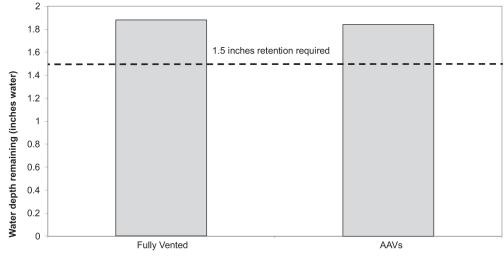
Figure 3. Comparison of water retained in the ground floor trap indicated (shaded on schematic)
