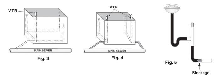
Note: Within each plumbing system a minimum of one stack vent or vent stack shall extend outdoors to open air. The stack vent or vent stack may be located anywhere within the system as long as it extends outdoors to open air.
