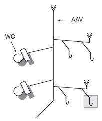
**Figure 2**. Two story house with AAVs on branches and an AAV termination at the top of the stack
