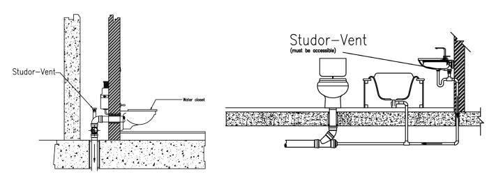
Terminating a waste stack on a Studor Single pipe system utilizing air admittance valves and P.A.P.A. devices.
