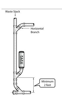
Stack extending no more than 5 floors above the base of the stack or offset should be a minimum of 2 feet
