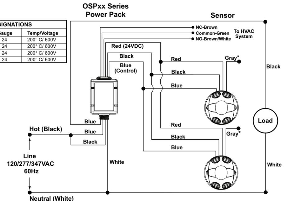
\*NOTE: When using the Photocell function, connect the Gray wire of the sensor to the Blue wire of the power pack. **DO NOT** use the Blue wire of sensor.
