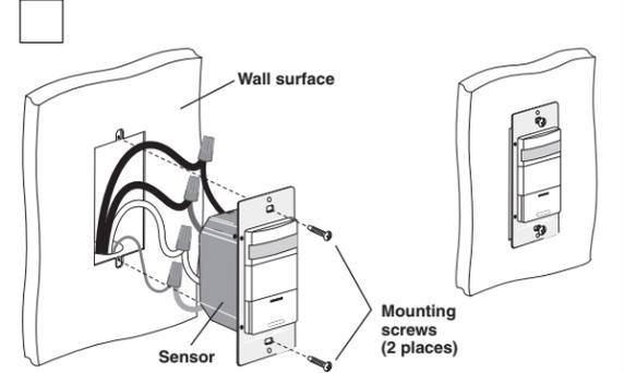
**NOTE:** Dress wires with a bend as shown in diagram to relieve stress when mounting device.
