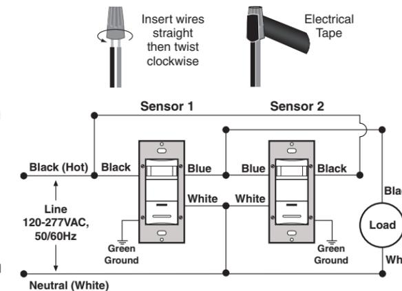
**NOTE:** Sensor 1 **must** be installed in a wall box that has both a LINE Hot and a Neutral connection. Sensor 2 **must** be installed in a wall box that has both a Load and a Neutral connection.
