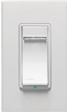
Vizia RF + 600W Electronic Low Voltage Scene Capable Dimmer for single pole, 3-way or more applications, with LED locator and brightness display. White face assembled on device, ivory and light almond faces included.
