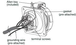
2. Mount. Mount (Table 5) and tighten mounting screws (Table 4).
