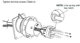
4 Mount Mount (Table 5) and tighten mounting screws.
