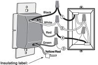
This wire is used in 3-way installations only For single pole installations, do not remove this insulating label.
