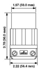
Mechanical Specifications Cord Range: .595 - .895 Product ID: Ratings and NEMA I.D. permanently marked on device Terminal Accom.: 18-10 AWG Terminal ID: Brass-Hot, Green-Ground, Silver-Neutral Wire Gauge: 14-10 AWG
