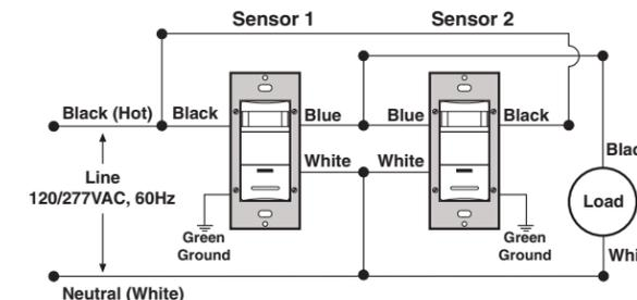
**NOTE:** Sensor 1 **must** be installed in a wall box that has both a LINE Hot and a Neutral connection. Sensor 2 **must** be installed in a wall box that has both a Load and a Neutral connection.
