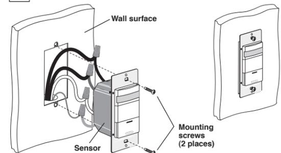
**NOTE:** Dress wires with a bend as shown in diagram to relieve stress when mounting device.
