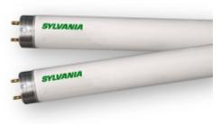
General28W, 48" MOL, T8 OCTRON Extended Performance Supersaver fluorescentDescription:lamp, 5000K color temperature, rare earth phosphor, 80 CRI, suitable for RS or<br/>IS operation, ECOLOGIC®3
