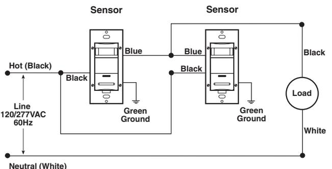
**NOTE:** Either Sensor can turn the lights ON. Either Sensor must time-out to OFF, or both manual buttons must be pressed for the lights to turn OFF.
