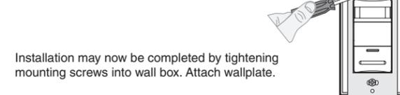
Installation may now be completed by tightening mounting screws into wall box. Attach wallplate.
