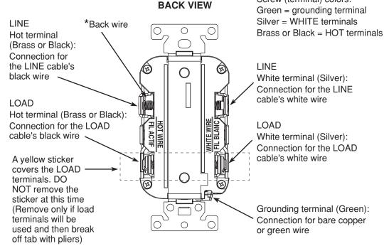
\* Back wire LINE terminals have a captive clamp feature to ease insertion of wires for first time wiring only.
