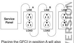
provide protection to "load side" receptacles B and C. On the other hand. placing the GFCI in position C will not provide protection to receptacles A or B. Remember that receptacles A, B, and C can be in different rooms.
