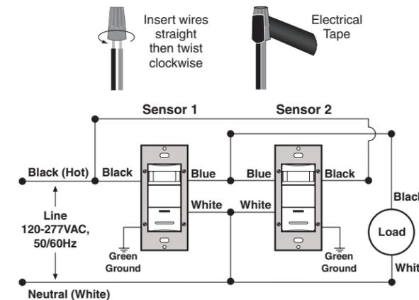
**NOTE:** Sensor 1 **must** be installed in a wall box that has both a LINE Hot and a Neutral connection. Sensor 2 **must** be installed in a wall box that has both a Load and a Neutral connection.
