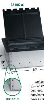
Boxes are shipped with disposable sheet metal cover to protect box during concrete pour. Box supplied with two  $1/2 - 3/4^{"}$  combination conduit knockouts each end for conduit feed and complete with four adjustable legs for prepour adjustment. Standard boxes supplied with power plates and data/communication plates punched to accept specified devices (see below).
