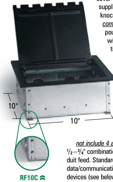
Boxes are shipped with disposable sheet metal cover to protect box during concrete pour. Box supplied with two 1/2-3/4" combination conduit knockouts each end for conduit feed and complete with four adjustable legs for pre-pour adjustment. Standard boxes supplied with power plates and data/communication plates punched to accept specified devices (see below).
