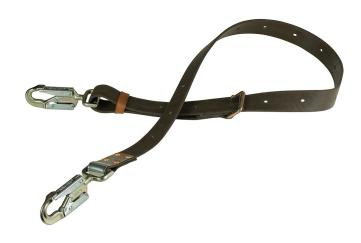
Klein's positioning straps work with Klein's climbing equipment for linemen. Made with exceptionally strong and long-lasting Klein-Kord, the straps are adjustable within a 2'3" range. Features a Gard snap hook with 5000 lb. (2268 kg) gate strength. The drop-forged, single tongue adjustment buckle has a corrosion-resistant finish. Depending on the application, choose a positioning strap that allows you to work at arm's length from the pole or other positioning anchorage.
