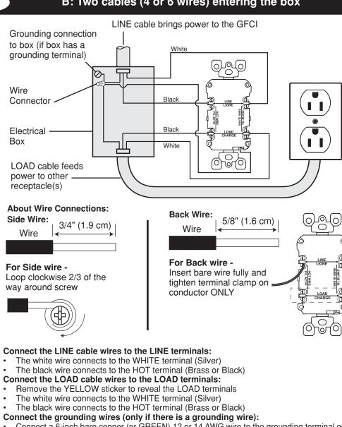
Connect a 6-inch bare copper (or GREEN) 12 or 14 AWG wire to the grounding terminal on the GFCI. If the box has a grounding terminal, also connect a similar wire to the grounding terminal on the box. Connect the ends of these wires to the LINE or LOAD cable's bare copper (or GREEN) wire using a wire connector. If these wires are already in place, check the connections.
