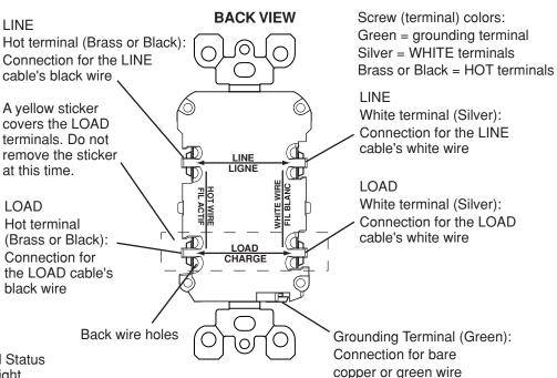
(a) Detach one cable's white wire and hot wires from the receptacle and cap each one separately with a wire connector. Make sure that they are from the same
