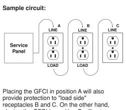
placing the GFCI in position C will not provide protection to receptacles A or B. Remember that receptacles A, B, and C can be in different rooms.
