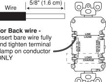
(a) This GFCI is shipped from the factory in the tripped condition and cannot be reset until it is wired correctly and power is supplied to the device. Plug a lamp or radio into the GFCI (and leave it plugged in). Turn the power ON at the service panel. Ensure that the GFCI is still in the tripped condition by pressing the TEST button. If the lamp or radio is OFF, and the GFCI will not reset, go to the
