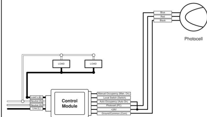
Photocell and Occupancy Sensor with Local Switch
