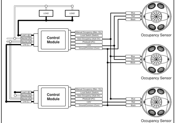
Multiple Loads Exceeding a Single Lighting Control Modules Load Rating
