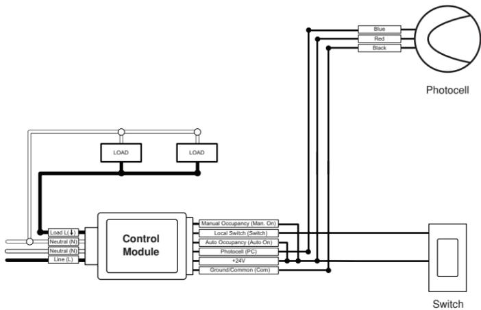
Multiple Occupancy Sensors Exceeding the Lighting Control Module Rating
