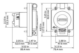
Mechanical Specifications Terminal Accom.: #16 AWG to #10 AWG
