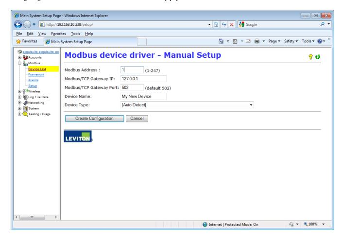
The manual setup page has several options that must be configured before the EMB HubLite will recognize the Modbus device. The options are as follows:
