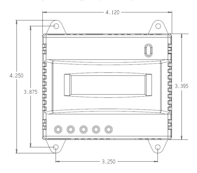
The EMB HubLite has 4 mounting holes for use with a #6 screw. The drawing above shows the relative position of the mounting holes.
