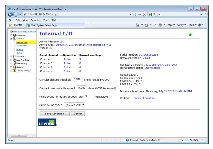
Specific options available in the Advanced Configuration page vary depending on the features available in the Modbus Device, as well as the features implemented in the built in EMB HubLite driver.
