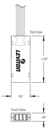
Fiber Optic Fanout Kits are available in six or twelve fiber capacity and in lengths of 24" or 36".
