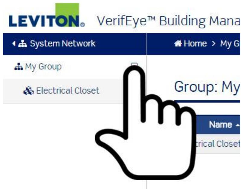
16. Click the plus sign next to the hub to view all meters connected to the hub.
