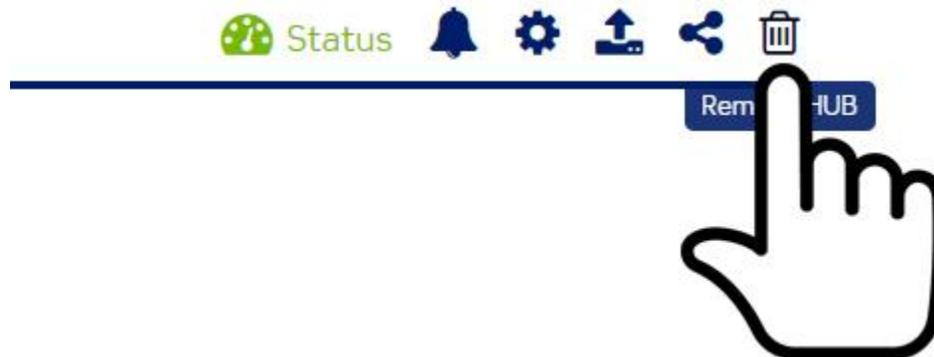
2. The remove hub screen is displayed. This option allows you to remove a hub from a group.
