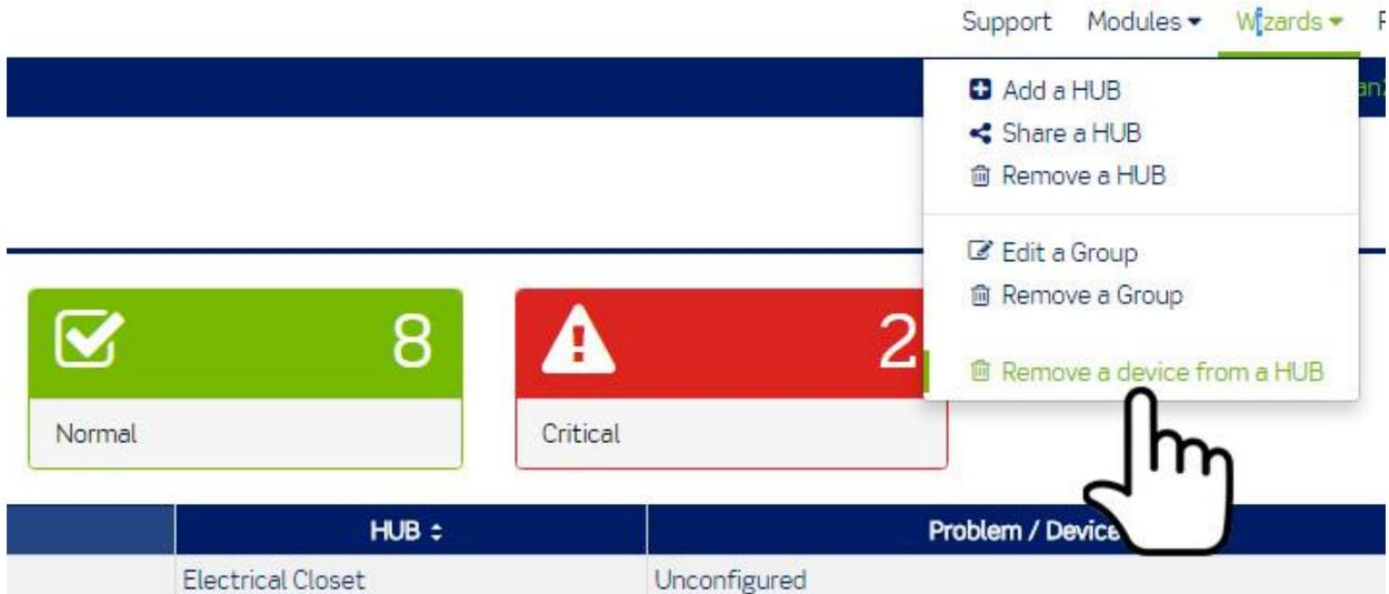
The remove device screen allows you to remove a device from a hub.
