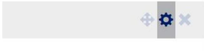
3. Remove widget. This control removes the widget from the executive dashboard. Note: Saved configuration settings are deleted with the widget.
