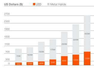
$^{\star}$  Based on 50,000 hours for LED replacement lamp compared to traditional HID technologies
