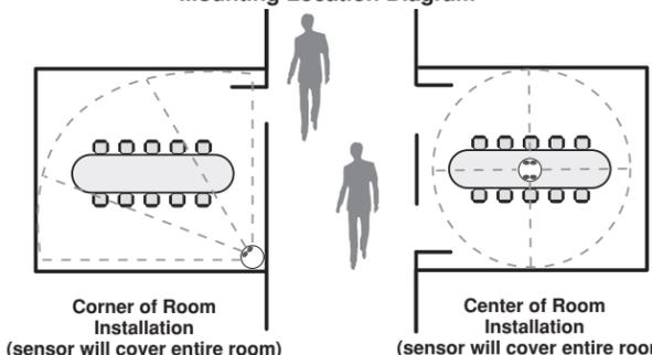
**NOTE:** When mounting device, do not point sensor openings towards the opening of a door or strong air currents.
