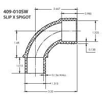
CA Title 24 Code: All elbows shall be sweep elbows or of an elbow type that has a pressure drop of less than the pressure drop of straight pipe with a length of 30 pipe diameters.
