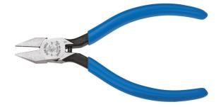
Klein Tools' 4-Inch Electronics Pliers offer added comfort for cutting applications that demand precision and control. Its sharp, pointed nose is designed for precise tip cutting and trimming of printed circuit boards. Spring-loaded cutting action and semi-flush cutting blades make this an essential tool for precision work.
