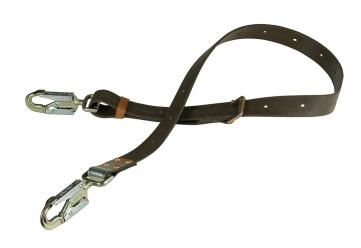
Klein's positioning straps work with Klein's climbing equipment for linemen. Made with exceptionally strong and long-lasting Klein-Kord, the straps are adjustable within a 2'6" range. Features a Gard snap hook with 5000 lb. (2268 kg) gate strength. The drop-forged, single tongue adjustment buckle has a corrosion-resistant finish. Depending on the application, choose a positioning strap that allows you to work at arm's length from the pole or other positioning anchorage.
