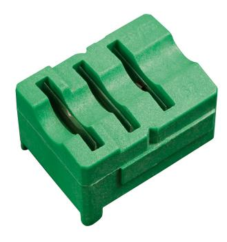
Designed for use with Klein's Radial Strippers. Three levels of blades stripRG58, RG59 and RG62 coax cable. Pre-set cutting blades save time and provide precise cutting. The cartridge is made from aglass filled polycarbonate for increased strength and durability.
