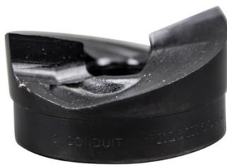
The 2.416-Inch Knockout Punch easily punches holes for 2-Inch conduit. It offers an optimized design that reduces wrench effort. Slugs are split inside for easy removal. Cuts aluminum, fiberglass and plastic as well.
