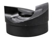
Easily punch holes for1-1/2-Inch EMT conduit. Has a maximum capacity of 10 gauge mild steel. Cuts aluminum, fiberglass and plastic as well. Optimized design reduces wrench effort. Slugs are split inside for easy removal.
