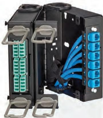
With a capacity of one SDX cassette or adapter plate — up to 24 LC fibers or 12 SC fibers — the Opt-X SDX Mini Wall-Mount Enclosure provides simple deployment and flexible mounting options for remote network hubs, non-traditional network areas, and other areas with extreme space constraints. It also accepts copper ports by using a QuickPort adapter plate (5F100-6QP).
