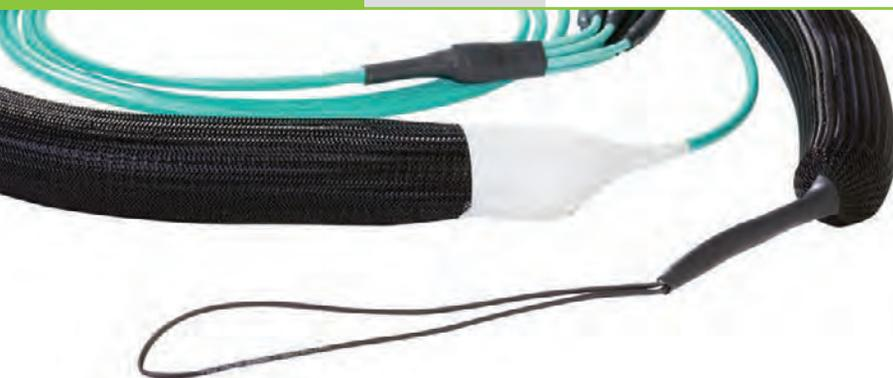
The pulling eye protects fiber connectors on 12- through 144-fiber trunk cables. It completely covers the breakout length, transferring any pulling force from the assembly to the pulling eye sleeve. Customers can specify which end to have the pulling eye installed.
