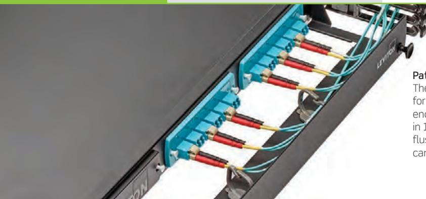
**Patch Cord Management Trays** help route and organize cables. The trays feature identification labels and front saddles that pivot for easier routing. Because they mount directly to the front of the enclosures, they do not require additional rack space. Available in 1RU and 2RU sizes, the trays can be used with any Leviton 1RU flush-mount MTP enclosure or e2XHD flat panel, and 2RU trays can be used with 3RU 500i SDX enclosures. **See page B22.**
