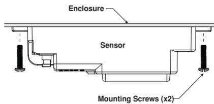
Fig. 3 (Flush mounting)
