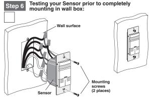
**NOTE:** Dress wires with a bend as shown in diagram to relieve stress when mounting device.
