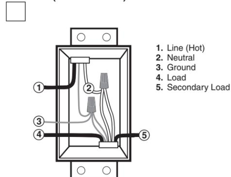
**Step 3** **Preparing and connecting wires:**
