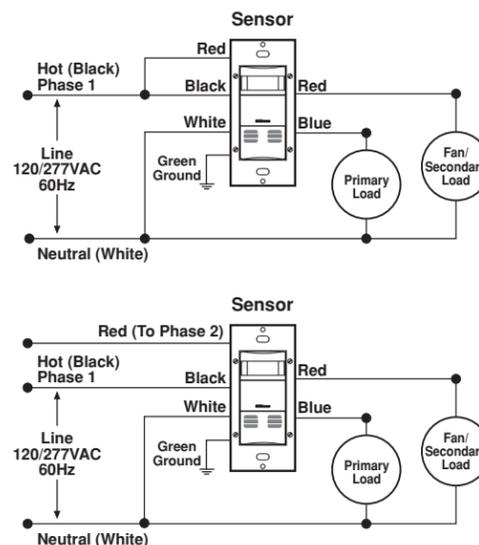
**Step 5** **Installing your Sensor - Multi-Location Wiring Application:**
