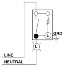
Mechanical Specifications Terminal ID: Brass-Hot, Green-Ground, Silver-Neutral Terminal Accom.: 14-12 AWG Termination: Side Wire
