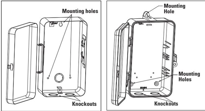
Position at eye level if possible, providing space to the left of the enclosure for the cover to swing open fully, as shown.
