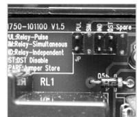
4. **ET8215C ONLY**—Decide whether you want to control multiple loads simultaneously (SIM), independently (IND), or with a 2-second pulse (PUL) (e.g., for use with mechanically held contactors or bell ringing applications), and make sure the jumper is positioned accordingly. See location **B** in *Rear View* above and detail at the right. (The unit is shipped with the loads set for IND.)
