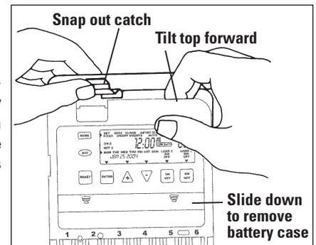
1. Remove the mechanism from the case by depressing the catch at the top of the case and pulling out, as shown.
