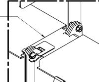
1485 FITTINGS FOR SIZES D & E (D - 6 X 6) AND (E - 8 X 8) PART # QTY DESCRIPTION DROP HANGER (BRACKET HANGER) 12 1/4 - 20 NUT 1/4 - 20 X 3/4 BOLT W/ NUT 1/4 - 20 X 1.5 BOLT W/ SEMS WASHERS
