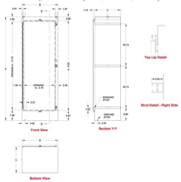
Note: 4 eyebolts are provided for 30.06" and 36.06" deep enclosures (both dual and single access)
