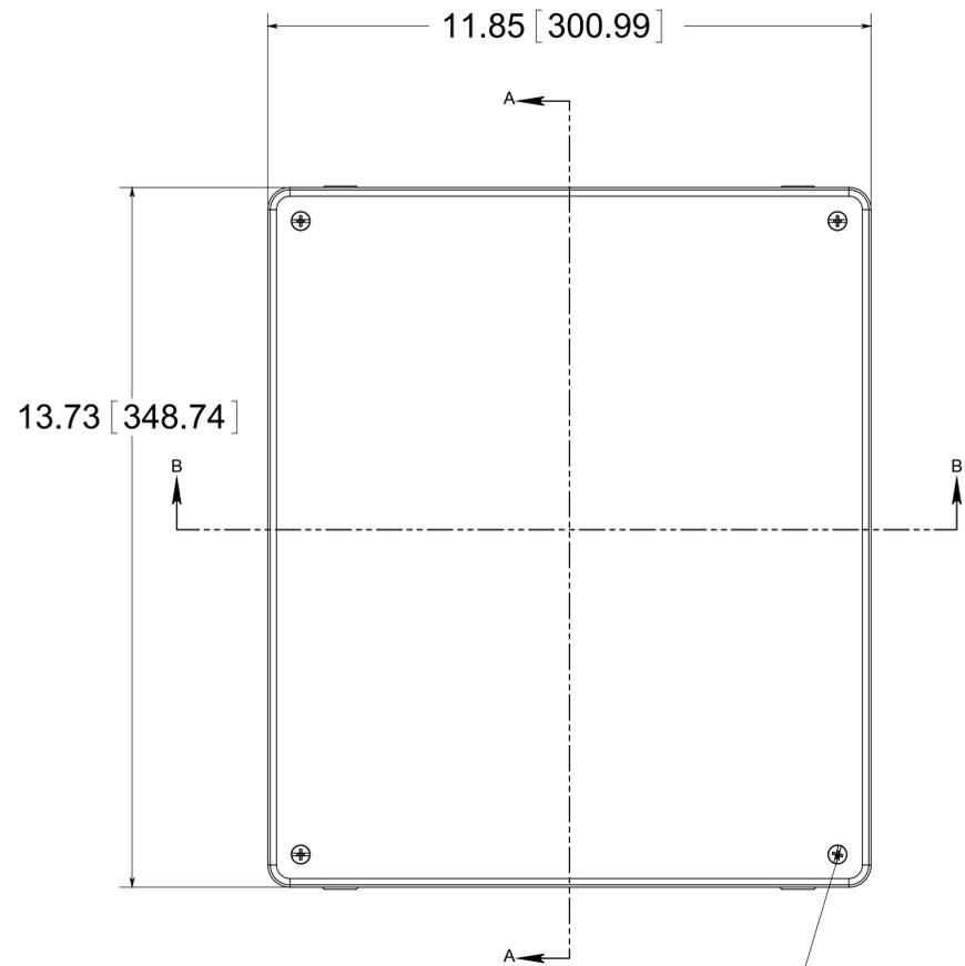
(4) EACH #10-32 BRASS INSERTS AND STAINLESS STEEL CAPTIVE COVER SCREWS WITH RETAINING O-RING
