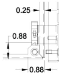
Retractable pin allows door to be mounted on left or right side
