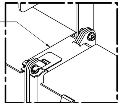
ASSEMBLED VIEW SHOWING SEALING PLATE
