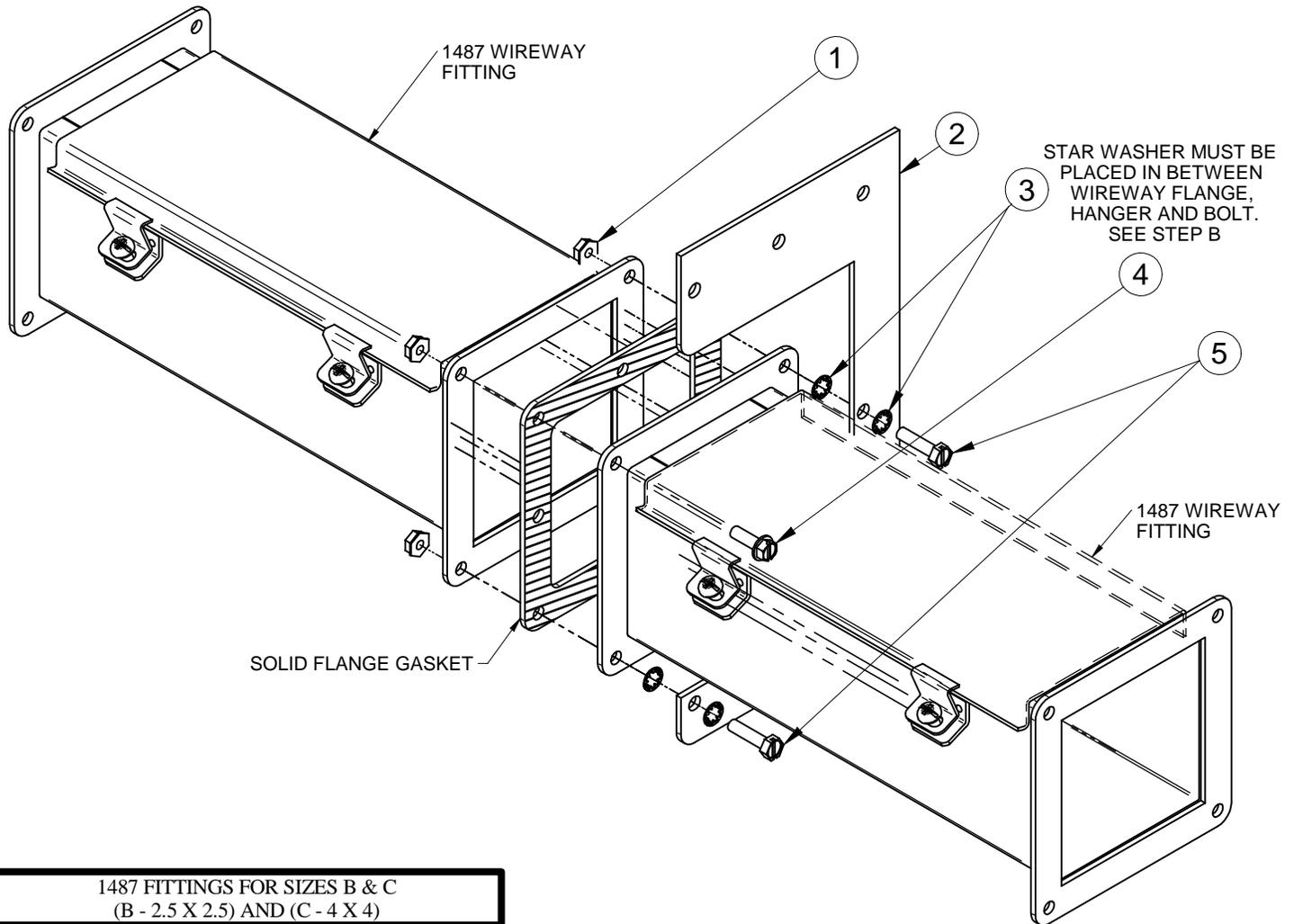
STAR WASHER MUST BE PLACED IN BETWEEN WIREWAY FLANGE, HANGER AND BOLT. SEE STEP B
